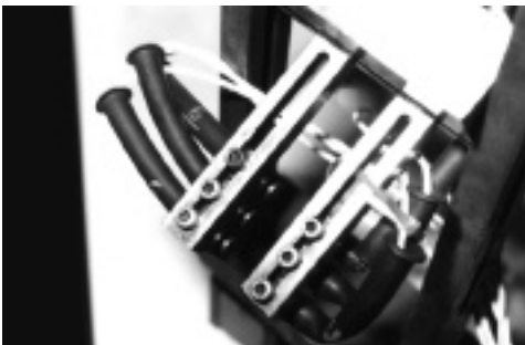
Close-up of probe holder, showing adjustable fixture used to adapt to different rotor sizes.
