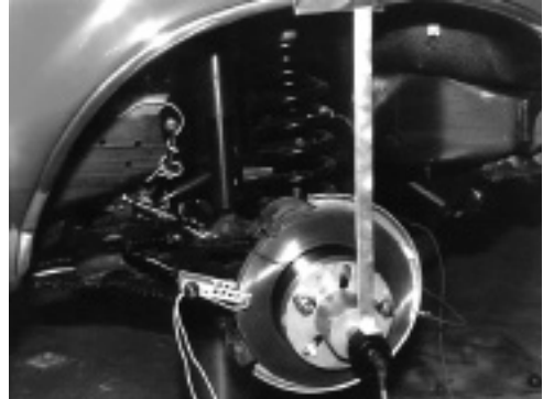
Capacitive probes mounted in a holder measuring disc brake wear and run out during on-vehicle testing.
