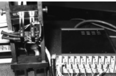
The capacitive probes mounted in a magnetic based fixture, shown with the associated signal conditioning amplifiers.
